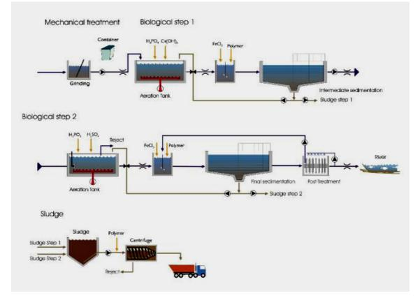
The wastewater flows from the tannery to the new inlet pumping station through a 2mm screen. The wastewater is then pumped to biological treatment as follows:
